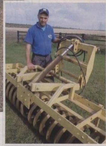
Wheeling problem solved: an extra press behind the plough and a front-mounted press on the drill tractor
