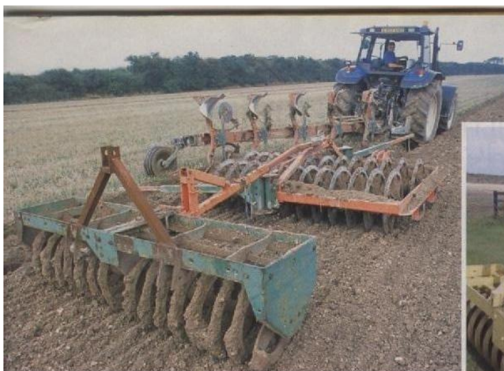
Wheeling problem solved: an extra press behind the plough and a front-mounted press on the drill tractor
