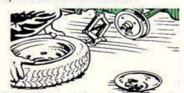
5: REMOVE lug nuts from wheel by turning them counterclockwise, and keep them in your hubcap so they don't roll away. Remove flat tire and lay flat. You don't want it to roll away either.
