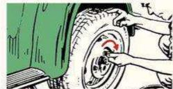
6: LINE UP spare tire with wheel studs and place on car. Once wheel is on, replace lug nuts and tighten them by hand, and then with your lug wrench, until you meet firm resistance.
