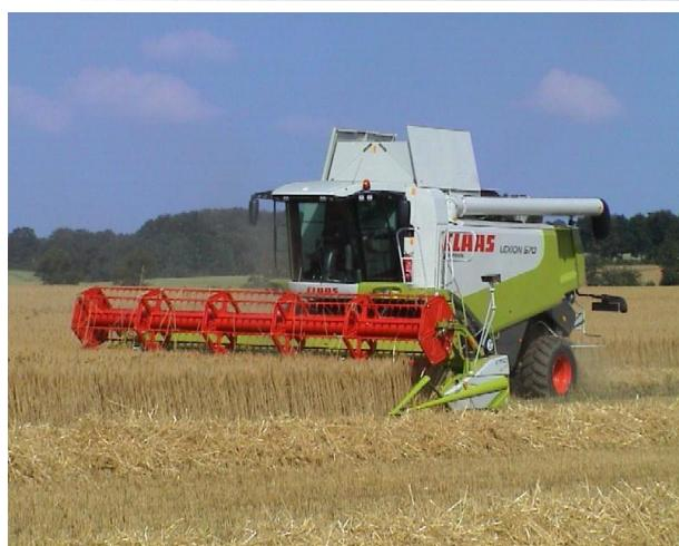
Harvesting oats in a Claas Lexion 570 combine with enclosed, air-conditioned cab with rotary thresher and laser-guided hydraulic steering
